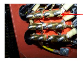
Remove ALL the brass jumper bars from ALL studs
