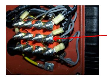
NOTE: ALL wires are to stay in existing locations. Remove <u>ALL 12</u> nuts from motor studs using 5/16" hex socket.
