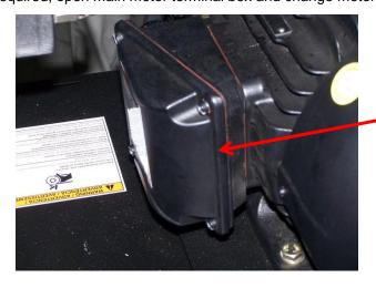
Remove motor cover using stubby screwdriver.
