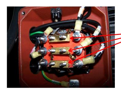
Install minimum 2 jumper bars across each horizontal 2 center studs. There should no other jumper bars on any other studs.
